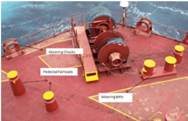
Figure 2 – Example of a typical modern mooring arrangement (Not the vessel in the report)
