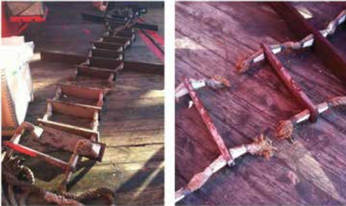
**Damaged pilot ladder on Platform Supply Vessel (Marine Safety Forum)**
