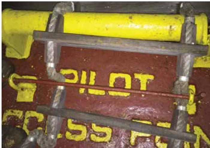
Figure 1 Steel bar used to secure ladder – not SOLAS compliant
