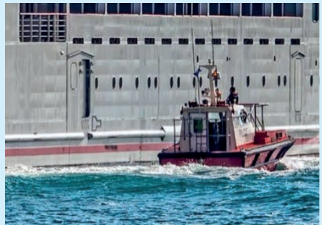
A new build passenger vessel with non-compliant SOLAS boarding arrangements
