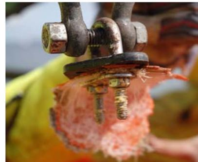
**CHIRP Narrative:** This Company report resonates with a previous report about a grp rescue boat in which the stainless steel bolts securing a lifting lug failed. In this recent case the grp material around the lifting eye failed. If you are aware of any incident with a rescue boat, please let us know.
